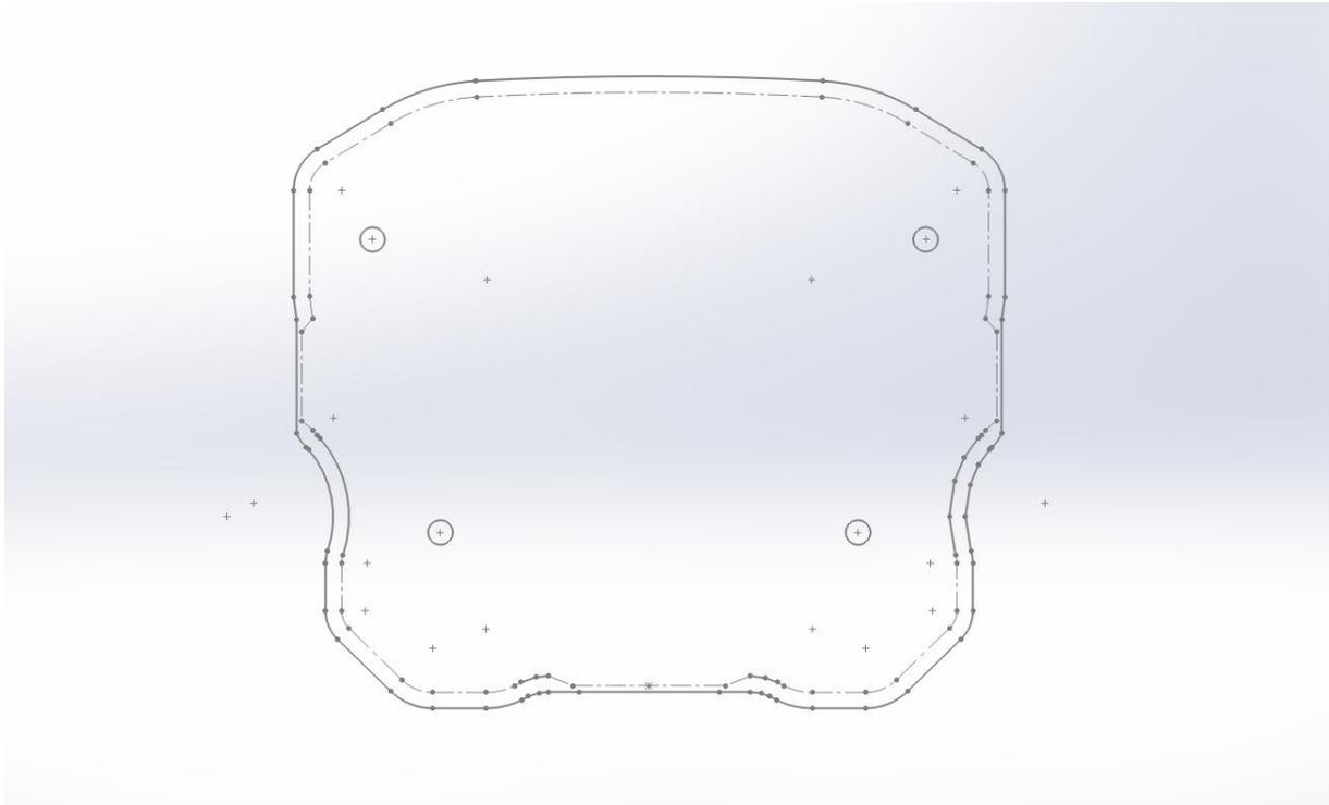
4 small circles represent mounting screws. Dashed inside line represents the available space where you can place your components and cutouts. When placing components, make sure that the mounting nut is also inside the dashed line.
